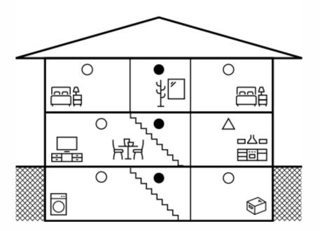
Smoke alarm devices for limited protection
