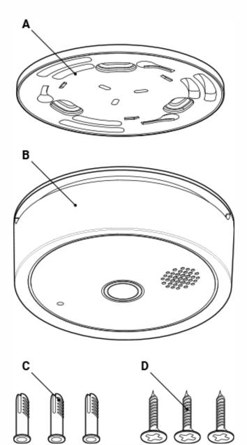
**A:** 1x mounting bracket **B:** 1x smoke alarm
