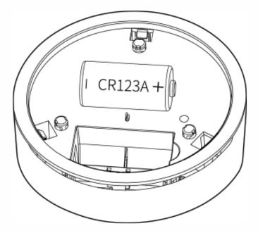
▲**CAUTION!** Replace only with the same or equivalent type! Danger of explosion if the battery is incorrectly placed.
