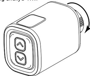
2. Fasten the Shelly® TRV to the radiator valve by turning the metal ring clockwise. Do not fully tighten the ring.
